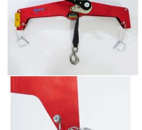
3. Slide out leg insert and attach in lowest hole
